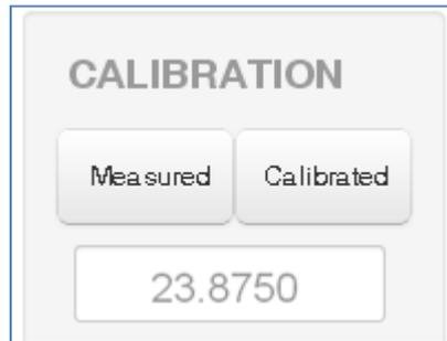
You can click on RAW and see the current value or you can write the theoretical value of the sensor output corresponding to the measurement.
