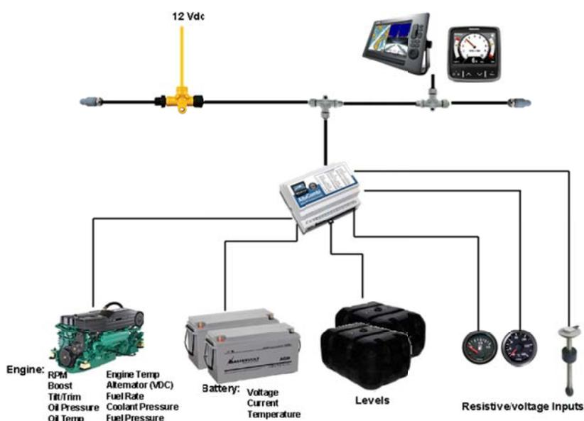
1. Select mounting location: Ensure the AlbaCombi can be mounted in a suitable location between the NMEA2000 bus and the senders or gauges.
