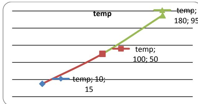
We assume that the sensor manufacturer indicates these values. In this way to 70 °C we must have a measure of 140 Ohms. You switch on the engine that you have 140 Ohms (you pressing on Measured until that value), then press “Calibrated” and see the value, if it is about 70°C, the calibration table is correct.
