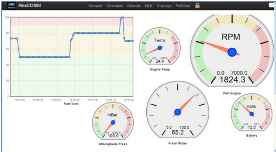
Press on the **padlock** icon to block/unlock the screen. In unlock mode you will can move the indicators.
