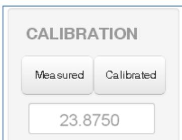
You can click on “Measured” and see the current value or you can write the theoretical value of the sensor output corresponding to the measurement.
